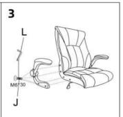
**NOTE**: Don't tighten the screws one by one. Try to align them first and tighten a few screws slightly. Then align the rest again and tighten them all.
