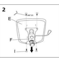
**NOTE**: The arrow points to the edge of the seat. (when you seat, the control handle is on your right hand side.)
