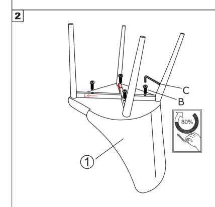
Put the chair onto flat place, fully tight all the screws after well adjusted flatness of the chair.
