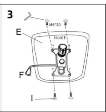
NOTE: Don't tighten the screws one by one. Try to align them first and tighten a few screws slightly. Then align the rest again and tighten them all.
